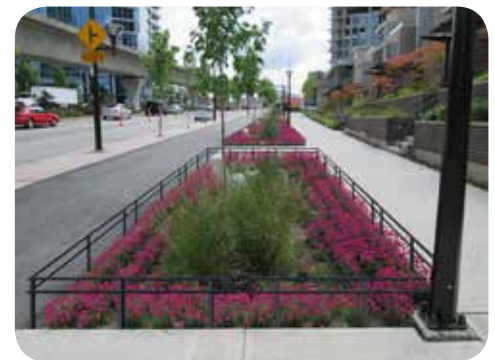
New Town Centre street standards with wide sidewalks, bicycle lanes, and rain gardens
