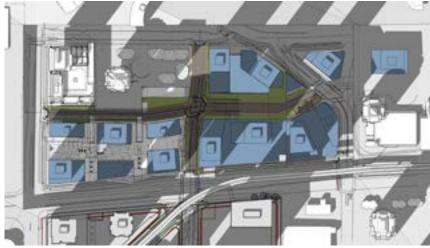
(FIGURE 6.13.3) JUNE SHADOW DIAGRAM AT 2:00 PM
