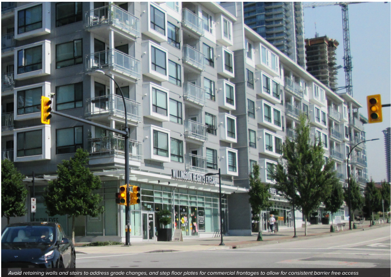
Avoid retaining walls and stairs to address grade changes, and step floor plates for commercial frontages to allow for consistent barrier free access
